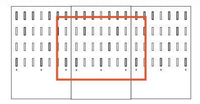
Determine the location on the wall where the opening in the Waterfall will be needed. Also determine the size of the opening required. Mark on wall exact cutout required. This may be completed by marking the wall directly, or by mounting a template made from paper or cardboard.
