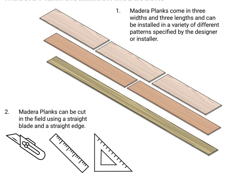
3. Madera Planks can be installed using either construction adhesive or a 23 ga. pin nailer.
